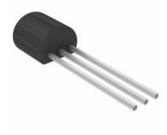
Wire a TMP36 temperature sensor to the first channel of an MCP3002 analog to digital converter and the other pins to +5V and GND
